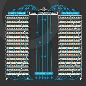
POWERFUL IMPELLER FANS DRIVE THE RE-CIRCULATED AIR TO THE FLOOR. CREATING NEGATIVE PRESSURE AT THE TOP OF THE CABINET.
