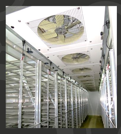
All corridor-based machines use the central corridor as what is effectively a pressure chamber to circulate air from the cooling/heating source throughout the lower racks and upwards in a circular fashion. Adequate vertical airflow is critical to uniformity. Heat transfer simply cannot occur if the air doesn't touch the egg, or is unable to carry air from the egg to the cooling/heating source for exchange.
