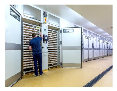
The PrimoTech™ comes fully equipped to the highest specification as standard, ensuring it performs to the maximum potential from day one. The paddle fan system and the hatcher's stainless steel interior walls being two such examples.
